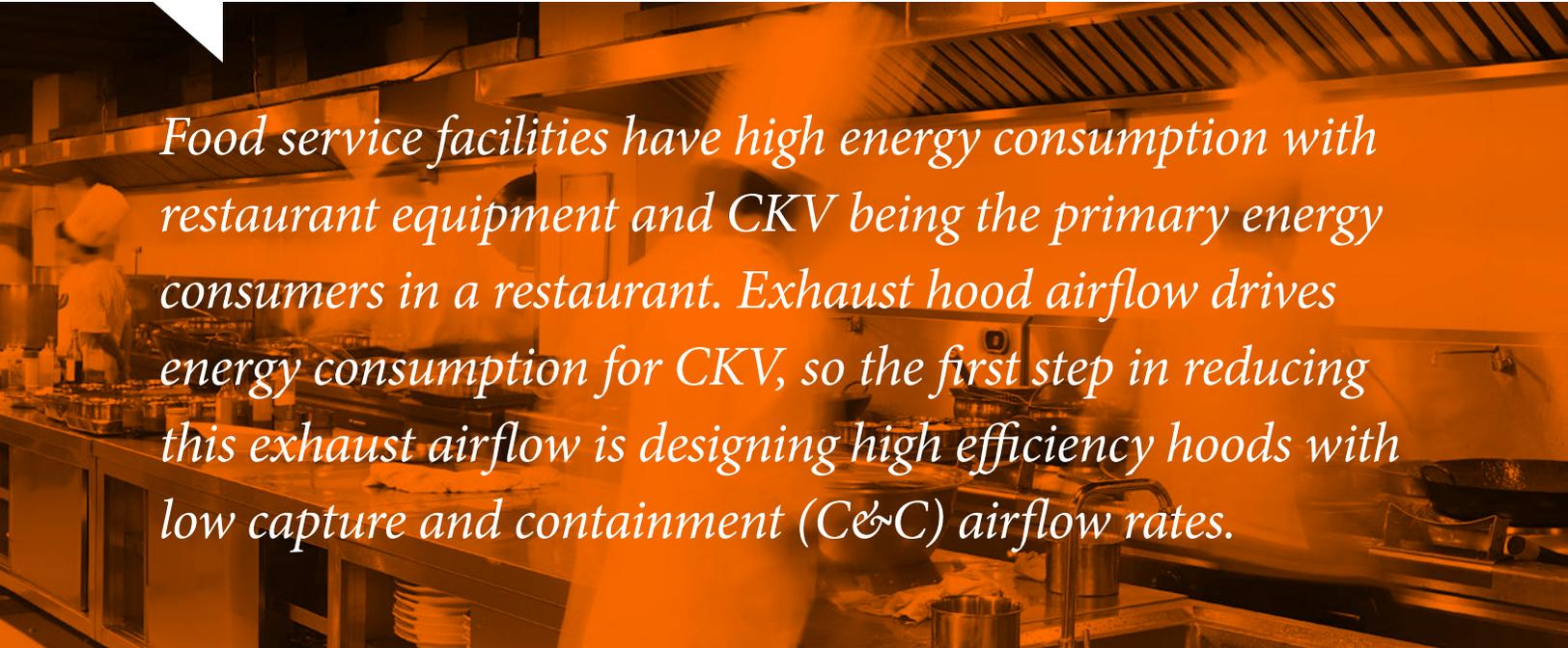
*Food service facilities have high energy consumption with restaurant equipment and CKV being the primary energy consumers in a restaurant. Exhaust hood airflow drives energy consumption for CKV, so the first step in reducing this exhaust airflow is designing high efficiency hoods with low capture and containment (C&C) airflow rates.*
